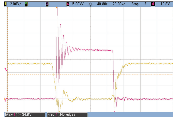
Figure 4: Typical waveforms for a 19V to 1.2V/15A (1 MHz) Buck converter CH1: Low side gate voltage – CH4: Switch node voltage
