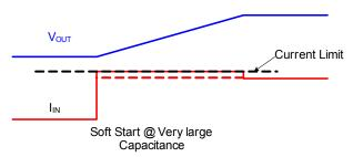
Figure 3: Soft Start Periods at different output capacitance
