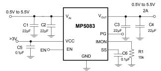
Figure 4: Typical Application Schematic
