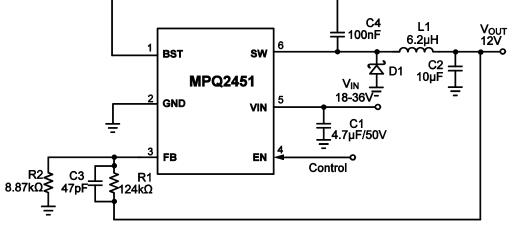
Figure 4: 12V Output Typical Application Schematic
