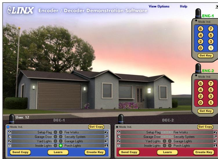
Figure 5: The Encoder / Decoder Demonstration Software Window in Software Operation Mode After Programming
