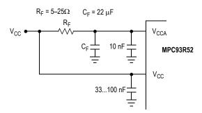
Figure 7. V<sub>CCA</sub> Power Supply Filter
