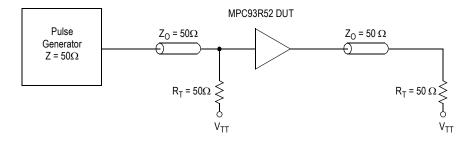
Figure 13. CCLK MPC93R52 AC Test Reference for V<sub>CC</sub> = 3.3 V and V<sub>CC</sub> = 2.5 V
