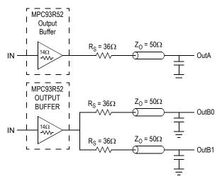
Figure 10. Single versus Dual Transmission Lines
