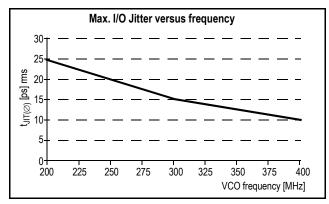
Figure 9. Max. I/O Jitter versus Frequency
