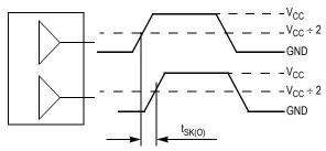
The pin-to-pin skew is defined as the worst case difference in propagation delay between any similar delay path within a single device
