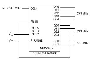
MPC93R52 zero-delay (feedback of QB0 = 33.3 MHz). Equivalent to Table 2 except F\_RANGE = 1 enabling a lower input and output clock frequency.
