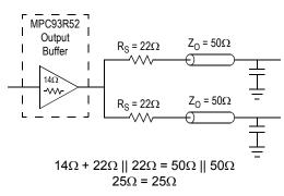
Figure 12. Optimized Dual Line Termination
