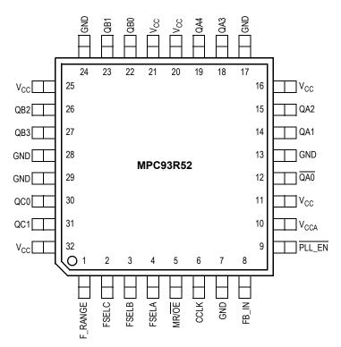
It is recommended to use an external RC filter for the analog power supply pin  $V_{CCA}$ . Please see application section for details.
