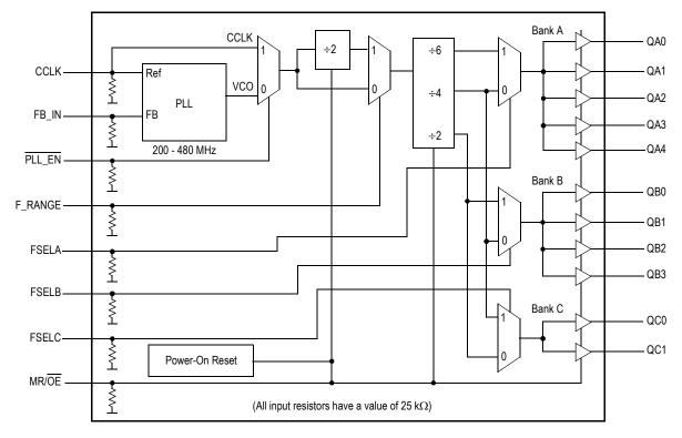
Figure 1. MPC93R52 Logic Diagram
