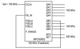
MPC93R52 default configuration (feedback of QB0 = 100 MHz). All control pins are left open.
