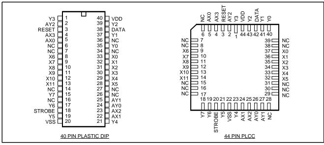
Figure 2 - Pin Connections
