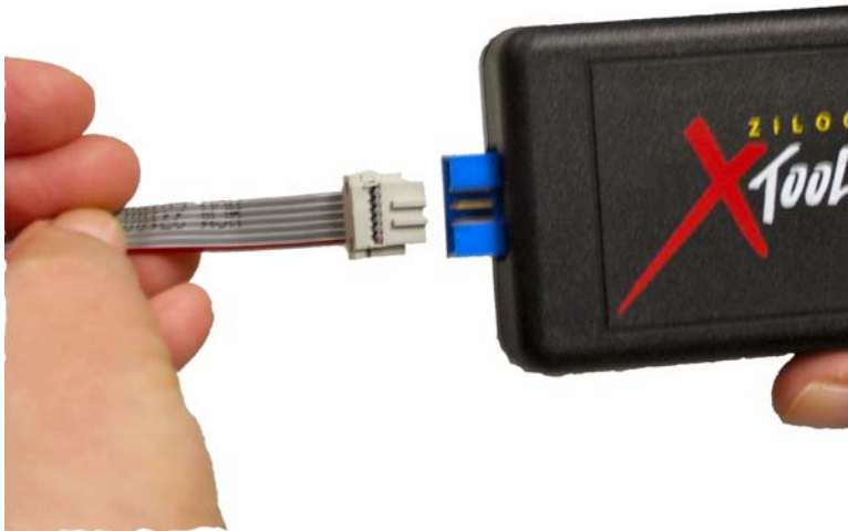
Figure 1. Connecting the Six-Conductor Ribbon Cable to the USB Smart Cable
