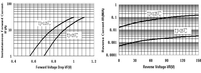
Fig.1-Typical Forward Voltage Drop Characteristics
