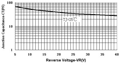
Fig.3-Typical Junction Capacitance Vs.Reverse Voltage
