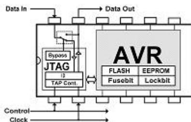
The FS2009(AVR-JTAG) supports programming of the Atmel ATmega AVR Microcontroller Family using the JTAG algorithm. This allows the FS2009 to program the ATmega devices at high speed via the JTAG port of the Target Device.
