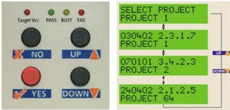
In 'Standalone Mode', the FS2009 is controlled via the push buttons on the front panel of the programmer - no PC connection is required. The programmer LCD and the LED Status Indicators are used to display the current status of the programmer. It is possible to select from 1 of 64 previously uploaded Programming Projects and then to repeatedly execute this project to program a batch of devices.
