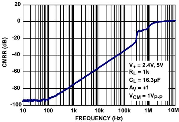
FIGURE 9. CMRR vs FREQUENCY,  $V_+ = 2.4V$  and  $5V$
