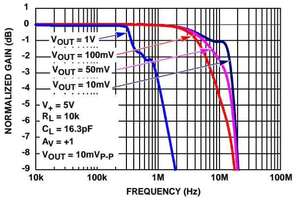
FIGURE 3. GAIN vs FREQUENCY vs  $V_{OUT}$ ,  $R_L = 10k$
