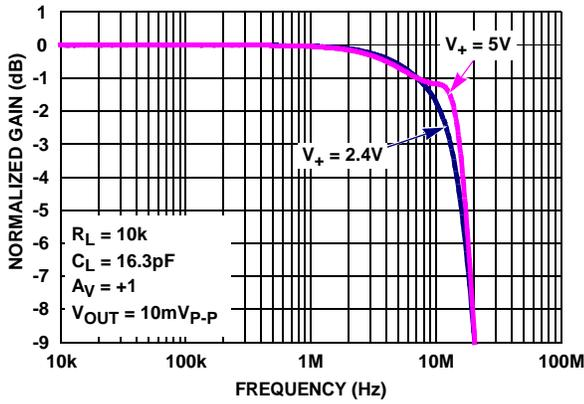
FIGURE 7. GAIN vs FREQUENCY vs SUPPLY VOLTAGE
