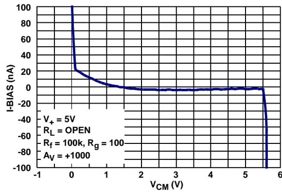
FIGURE 19. INPUT OFFSET CURRENT vs COMMON-MODE INPUT VOLTAGE
