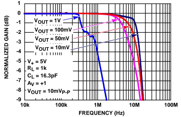
FIGURE 2. GAIN vs FREQUENCY vs  $V_{OUT}$ ,  $R_L = 1k$
