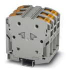
High-current terminal block, Blocked, Connection method: Power-Turn connection, Cross section: 10 mm<sup>2</sup> - 70 mm<sup>2</sup>, AWG: 8 - 2/0, Width: 60 mm, Color: gray, Mounting type: NS 35/15
