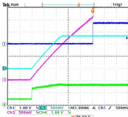
Figure 8. Typical Start-up Waveforms
