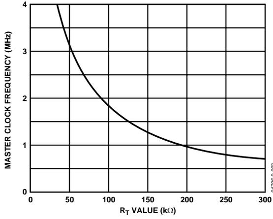
Figure 6. Master Clock Frequency vs. R<sub>T</sub>
