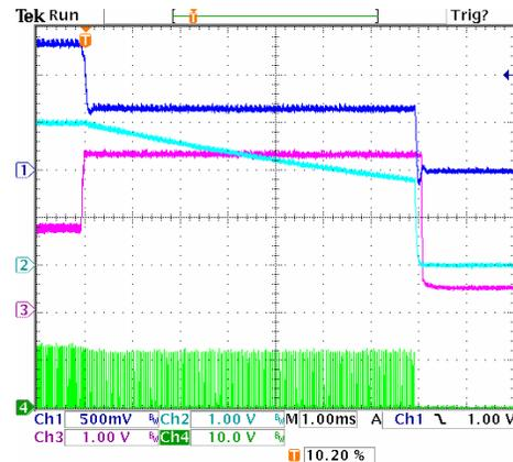
Figure 9. Overcurrent Latch-off Waveforms
