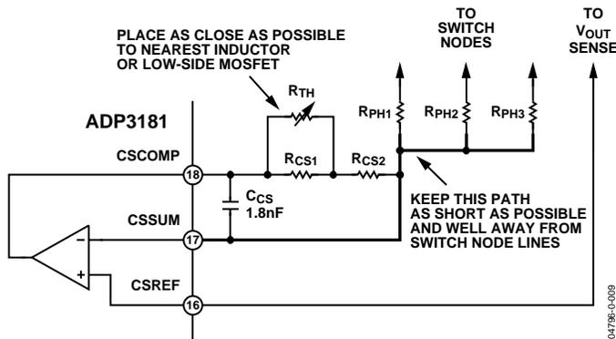
Figure 11. Temperature Compensation Circuit Values
