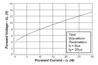
Fig3. Forward Voltage vs.Forward Current
