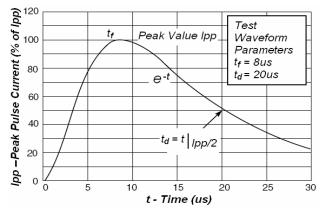
Fig1. Pulse Waveform
