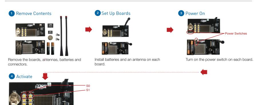
Push S0 to activate buzzer and push S1 to turn on the LED.
