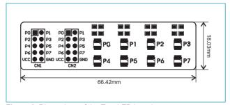
Figure 2: Dimensions of the EasyLED board
