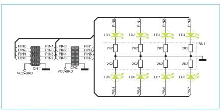
Figure 3: The EasyLED board connection schematic
