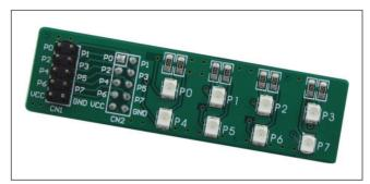
Figure 1: EasyLED additional board
