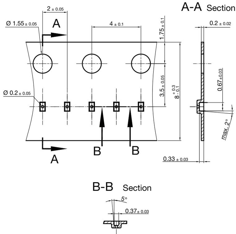
Cummulative tolerances of 10 sprocket holes is +/-0.2mm
