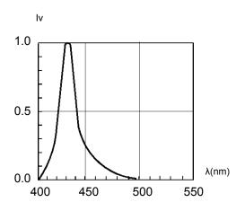
Fig. 1 Relative Luminous Intensity vs. Wavelength
