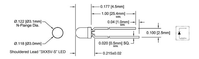
Recommended Mounting Hole Size = Ø.032<sup>+.003</sup><sub>-.002</sub>
