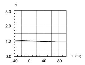
Fig. 3 Relative Luminous Intensity vs. Temperature
