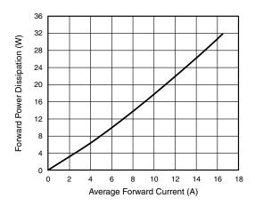
Fig. 3 - Forward Power Dissipation
