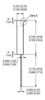
Polarity shown on front side of case, positive lead beveled corner
