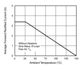
Fig. 2 - Forward Current Derating Curve
