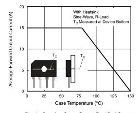
Fig. 1 - Derating Curve Output Rectified Current
