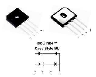
\* Tested to UL standard for safety electrically isolated semiconductor devices. UL 1557 4th edition. Dielectric tested to maximum case, storage and junction temperature to 150 °C to withstand 1500 V. Epoxy meets UL 94 V-0 flammability rating.
