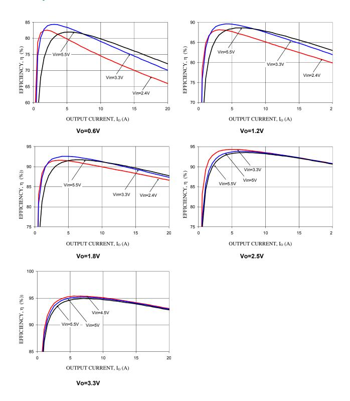
2.4 Vdc - 5.5 Vdc Input, 0.6 Vdc - 3.63 Vdc /20 A Output
