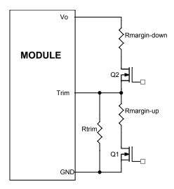
Circuit Configuration for margining Output voltage
