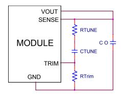
Circuit diagram showing connection of  $R_{\text{TUNE}}$  and  $C_{\text{TUNE}}$  to tune the control loop of the module
