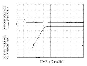
Start-up Using On/Off Voltage (Io = Io,max), Vo=1.8V
