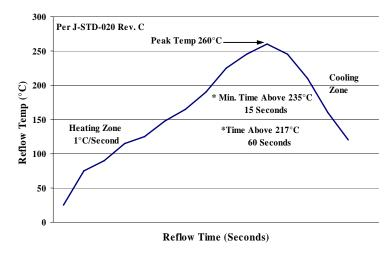
Recommended linear reflow profile using Sn/Ag/Cu solder
