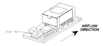
2.4 Vdc - 5.5 Vdc Input, 0.6 Vdc - 3.63 Vdc /20 A Output
