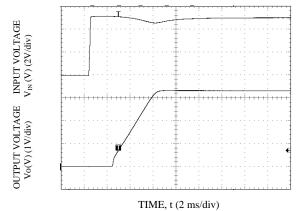
Start-up Using Input Voltage ( $V_{IN} = 5V$ ,  $I_0 = I_{o,max}$ ), Vo=3.3V
