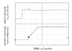
Start-up Using Input Voltage ( $V_{IN} = 3.3V$ ,  $I_o = I_{o,max}$ ),  $V_o=1.2V$
