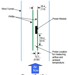
Thermal Test Setup
