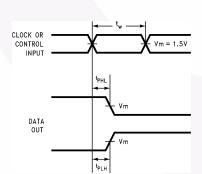
Figure 5. Propagation Delay, Pulse Width Waveforms
