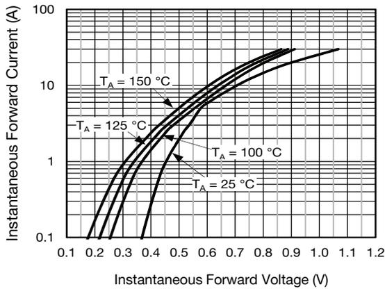
Fig. 3 - Typical Instantaneous Forward Characteristics Per Diode
