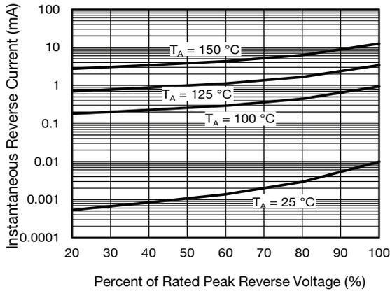
Fig. 4 - Typical Reverse Characteristics Per Diode
