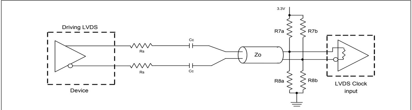
**Driving LVDS inputs with the PI6CFGL202B**
