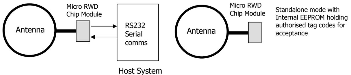
Remote mode (connected to a host computer or microcontroller) and Standalone mode.
