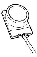
The Snap-in Legend Plate is easily removed by pressing the Snap-in Legend Plate from the back of the Legend Plate Frame.
