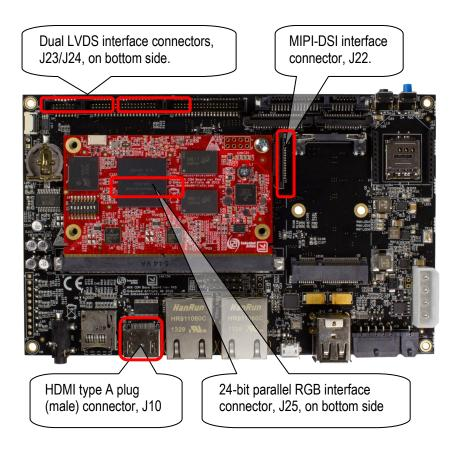
Figure 3 - Display Interfaces on COM Carrier Board
