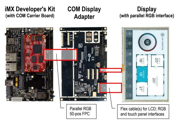
Figure 4 – Display Adapter Board Connection
