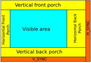
Name hannstar Pixel format 18 = RGB666 Pixel clock 64998375Hz 1024x768 Resolution 220 Horizontal back porch Horizontal front porch 40 Vertical back porch 21 7 Vertical front porch **Horizontal Sync** 60 **Vertical Sync** 10 0 (= active low) H-Sync active high/low V-Sync active high/low 0 (= active low) Display enable active 1 (= active high) Pixel clock data driven 0 (= falling edge)
