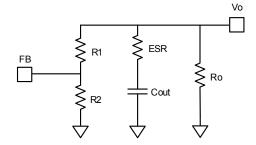
Figure 8—Simplified Circuit in skip Mode
