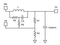
Figure11—Simplified Circuit of Ceramic Capacitor
