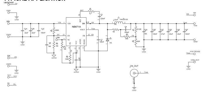
Figure 14 — Typical Application Circuit with Low ESR Ceramic Output Capacitor  $V_{IN}$ =6.5-22V,  $V_{OUT}$ =1.05V,  $I_{OUT}$ =6A
