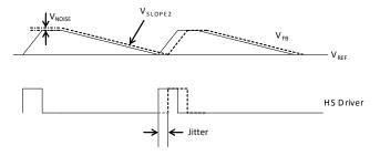
Figure 5—Jitter in Skip Mode
