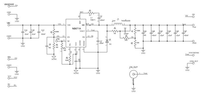
Figure 15 — Typical Application Circuit with Low ESR Ceramic Output Capacitor V<sub>IN</sub>=7-22V, V<sub>OUT</sub>=5V, I<sub>OUT</sub>=6A
