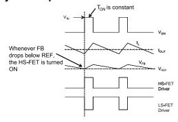
Figure 2—Heavy Load Operation
