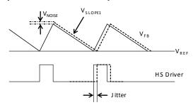
Figure 4—Jitter in PWM Mode
