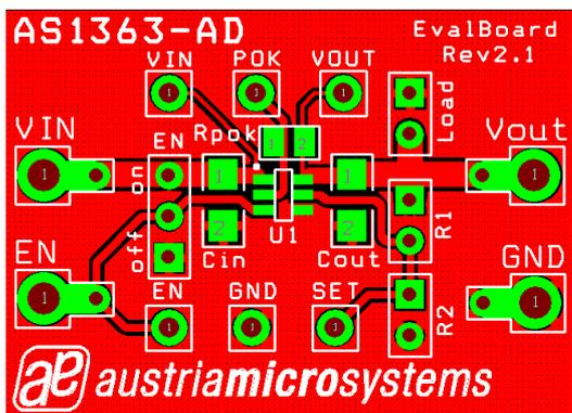
Figure 6: Top + Bottom Layer (adjustable Vout)
