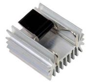
Ohmite's R2 Series (patent pending) heatsink provides a large surface area along with our C Series clipping mechanism to attach to a TO-220, TO-247, or TO-264 package. The self-aligning features of the clip assure secure attachment and enhanced thermal performance. Because no screws are required for device mounting, additional fins can be added to the rear side of the heatsink for increased total surface area in a more compact space.
