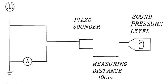
S.P.L. Measuring Circuit Input Signal: 10 Vp-p, 4.5 KHz, square wave Mic: RION S.P.L. meter UC30 or equivalent S.G.: Hewlett Packard 33120A function generator or equivalent
