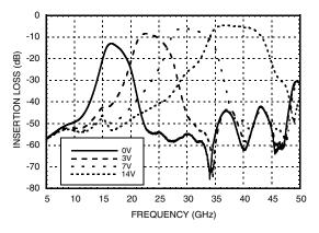
Insertion Loss vs. Vfctl
