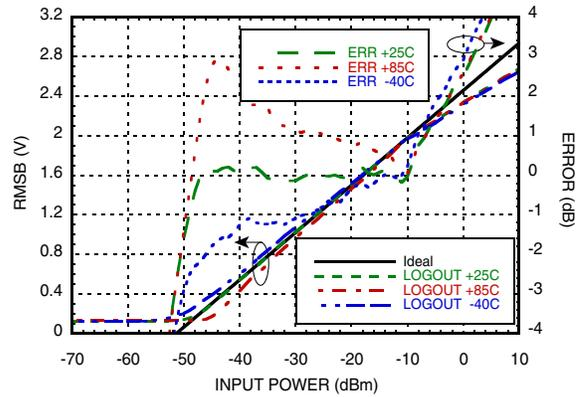
**OUT [P,N] & Error vs. Pin @ 100 MHz [1][2]**
