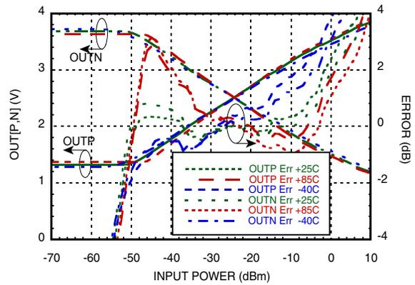
**OUT [P,N] & Error vs. Pin @ 3900 MHz [1][2]**
