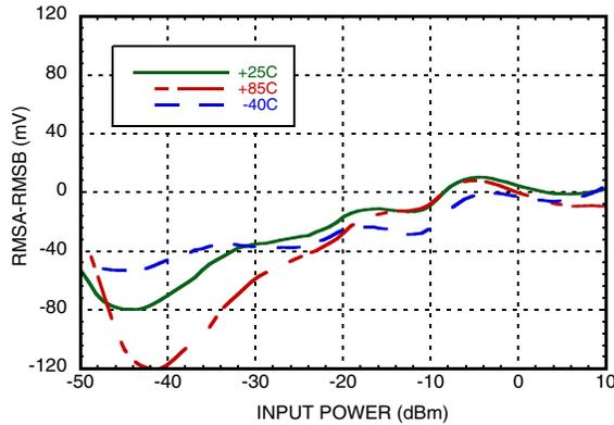
**RMSA-RMSB, Channel Matching vs. Pin over Temperature @ 3900 MHz [1] [2]**
