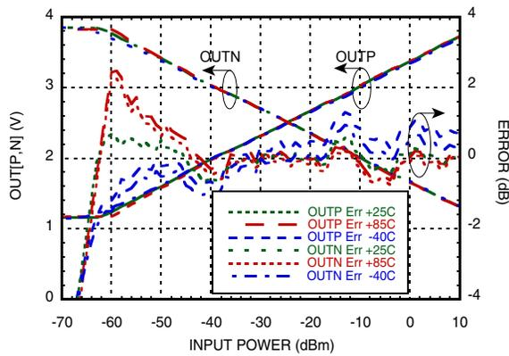
**OUT [P,N] & Error vs. Pin @ 900 MHz [1][2]**
