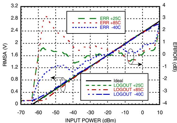
**RMSB & Error vs. Pin @ 1900 MHz [1]**
