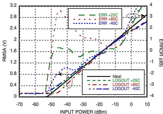
**RMSB & Error vs. Pin @ 3500 MHz [1]**
