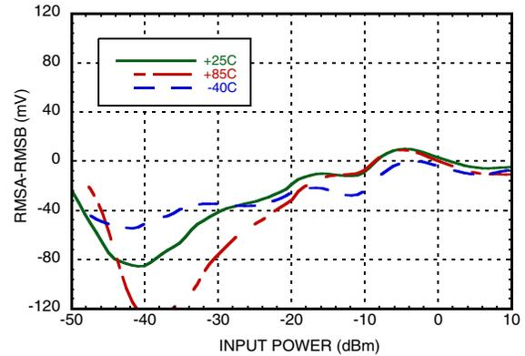
**Interference to an Input Signal (INB Power Fixed) with Interfering Signal on the other Channel (INA Power Swept) [1]**
