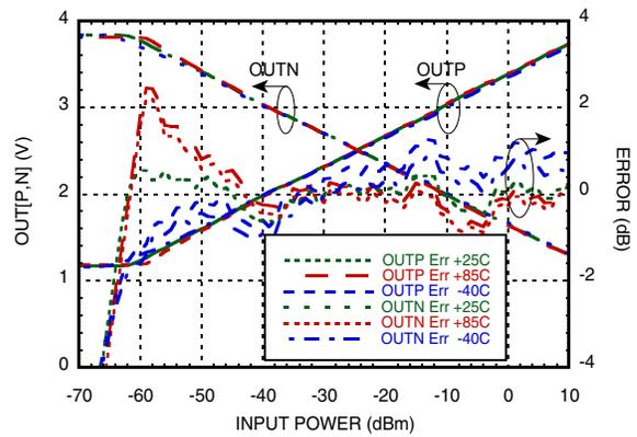
**OUT [P,N] & Error vs. Pin @ 1900 MHz [1][2]**
