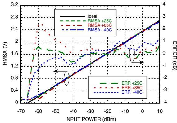
**RMSB & Error vs. Pin @ 100 MHz [1]**
