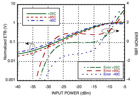
**ETA vs. Pin with CW @ 3500 MHz**
