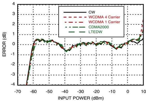
**RMSB Error vs. Pin with Different Modulations @ 1900 MHz<sup>[1]</sup>**
