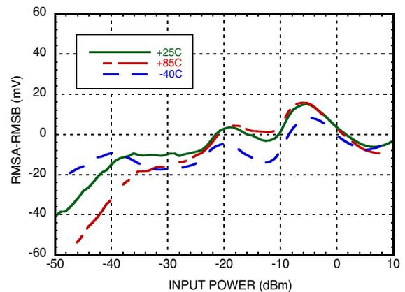
**RMSA-RMSB, Channel Matching vs. Pin over Temperature @ 2200 MHz [2] [3]**
