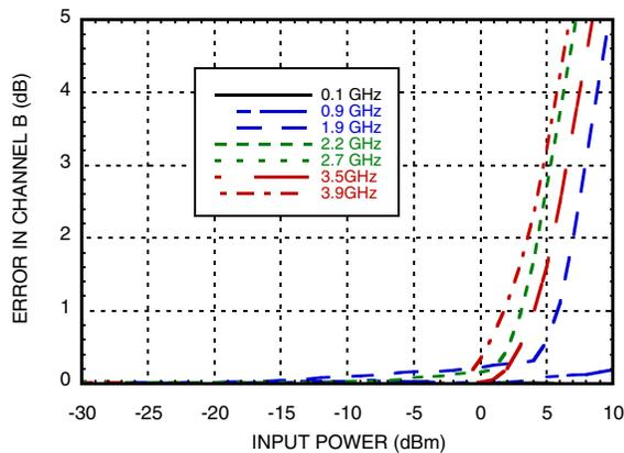
**Interference to an Input Signal (INA Power Fixed) with Interfering Signal on the other Channel (INB Power Swept)**
