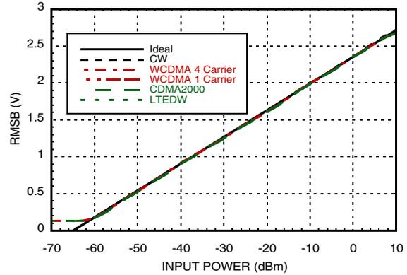
**RMSA Error vs. Pin with Different Modulations @ 1900 MHz<sup>[1]</sup>**
