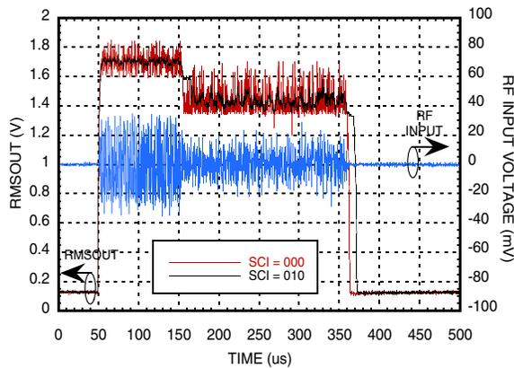
**Residual Ripple for 0.9 GHz WiMAX
