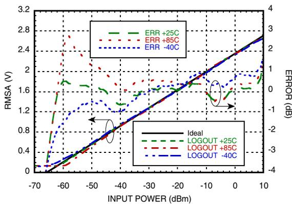
**RMSB & Error vs. Pin @ 900 MHz [1]**
