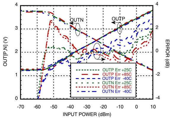
**OUT [P,N] & Error vs. Pin @ 3500 MHz [1][2]**
