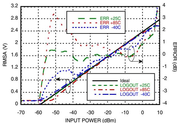
**RMSB & Error vs. Pin @ 2700 MHz [1]**
