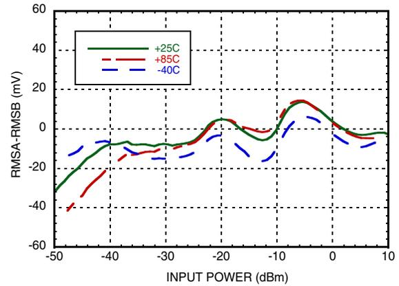
**RMSA-RMSB, Channel Matching vs. Pin over Temperature @ 900 MHz [2] [3]**
