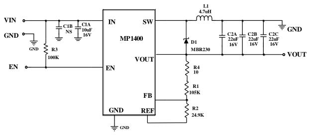
Figure 3: 5V<sub>IN</sub>, -5V/0.6A Output
