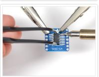
Once you've identified which is pin 1, hold the chip with the tweezers over the pads and then *re-heat* the corner pad you soldered onto a few steps ago.
