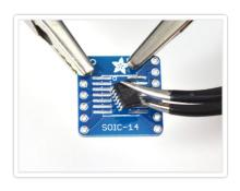
Next you need to place the part onto the pads, and you'll want to get the orientation right. You can look for a dot (indicating pin #1). In some cases, look for a flattened corner (on the left side here) which indicates which side is on the left
