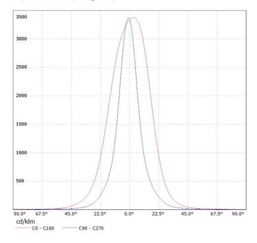
Luminaire: LEDIL OY CA11053-TINA2-O (NVS19) Efficiency=85% Lamps: 1 x Nichia NVS19 (98.3Im @ 250mA)
