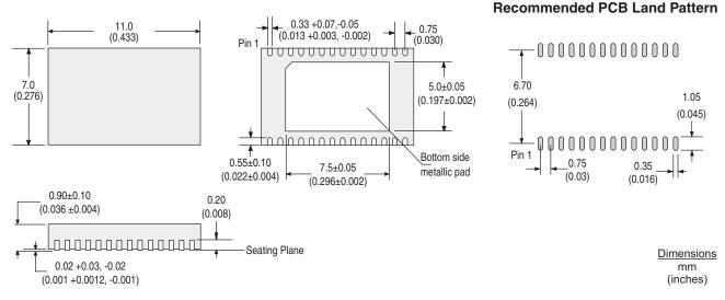
NOTE: Because the metallic pad on the bottom of the DFN package is connected to the substrate of the die, IXYS Integrated Circuits Division recommends that no printed circuit board traces cross this area to avoid potential shorting issues.
