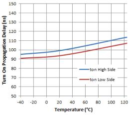
Figure 5. Turn-on Propagation Delay vs. Temperature
