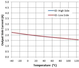
Figure 19. Output Sink Current vs. Temperature
