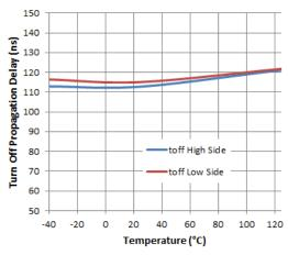
Figure 7. Turn-off Propagation Delay vs. Temperature
