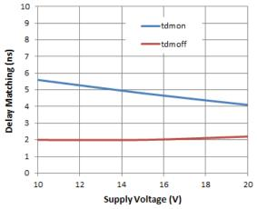
Figure 14. Delay Matching vs. Supply Voltage
