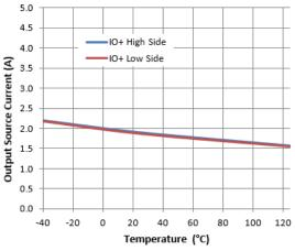
Figure 17. Output Source Current vs. Temperature
