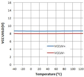
Figure 24. VCC UVLO vs. Temperature
