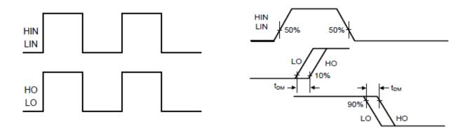
Figure 1. Input / Output Timing Diagram
