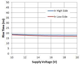
Figure 8. Rise Time vs. Supply Voltage
