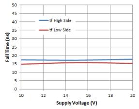
Figure 10. Fall Time vs. Supply Voltage
