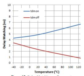
Figure 15. Delay Matching vs. Temperature
