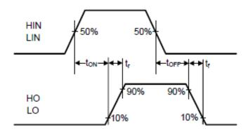
Figure 3. Switching Time Waveform Definitions
