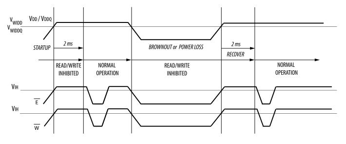
Figure 2.1 Power Up and Power Down Diagram
