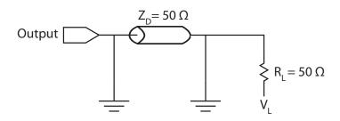
**Figure 3.2 Output Load Test All Others**
