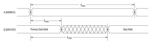
NOTE: Device is continuously selected  $(\overline{E} \le V_{\parallel}, \overline{G} \le V_{\parallel})$
