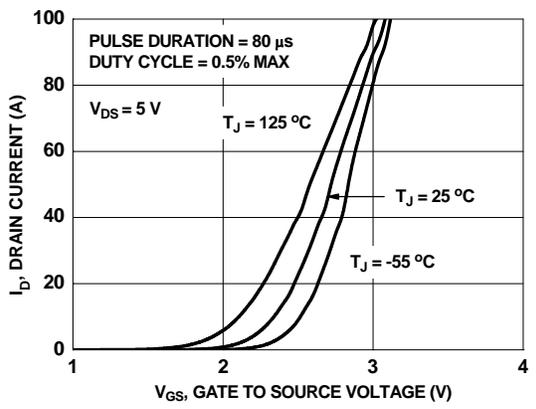
**Figure 5. Transfer Characteristics**
