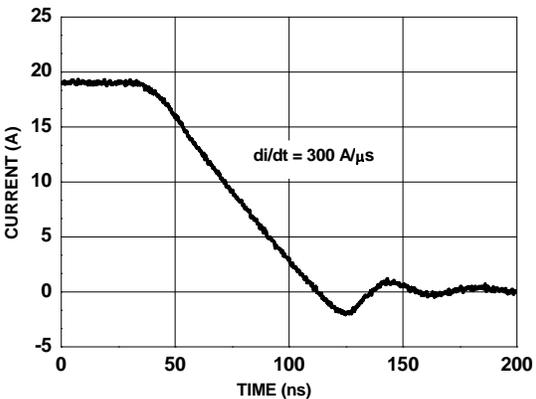
**Figure 14. FDMS0310AS SyncFET<sup>™</sup> body diode reverse recovery characteristic**
