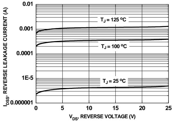
**Figure 15. SyncFET<sup>™</sup> body diode reverse leakage versus drain-source voltage**
