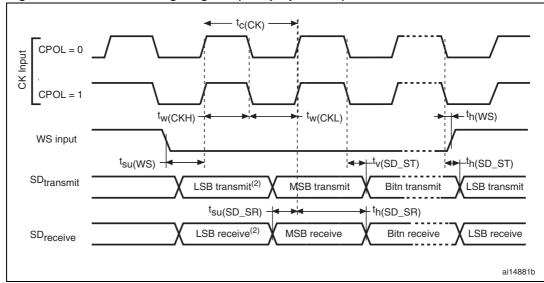
Figure 27. I<sup>2</sup>S slave timing diagram (Philips protocol)<sup>(1)</sup>
