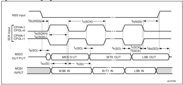
1. Measurement points are done at 0.5V  $_{\rm DD}$  level and with external C  $_{\rm L}$  = 30 pF.
