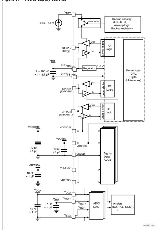
Dotted lines represent the internal connections on low pin count packages, joining the dedicated supply pins.
