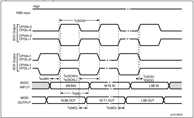
1. Measurement points are done at  $0.5V_{DD}$  level and with external  $C_L$  = 30 pF.
