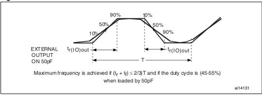
Figure 21. I/O AC characteristics definition
