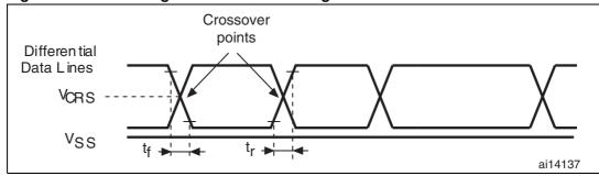
Figure 32. USB timings: definition of data signal rise and fall time
