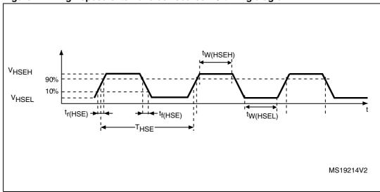
Figure 12. High-speed external clock source AC timing diagram
