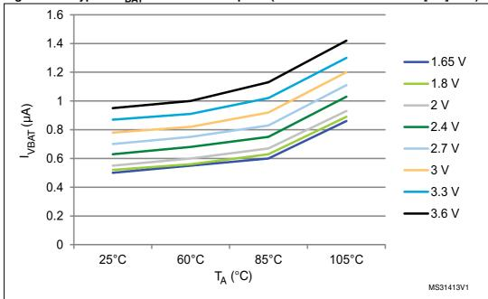
Figure 11. Typical V<sub>BAT</sub> current consumption (LSE and RTC ON/LSEDRV[1:0]='00')
