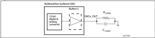
The DAC integrates an output buffer that can be used to reduce the output impedance and to drive external loads directly
