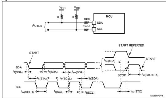
1. Measurement points are done at CMOS levels:  $\rm 0.3V_{DD}$  and  $\rm 0.7V_{DD}.$
