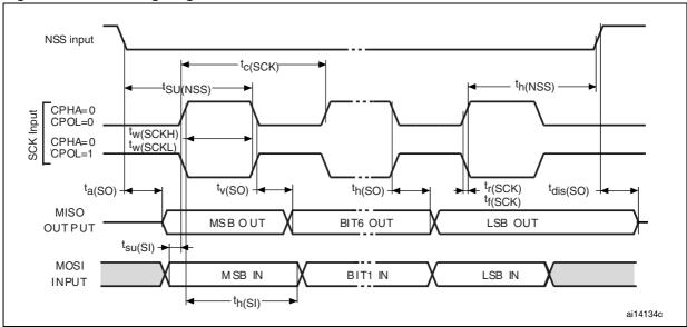
Figure 25. SPI timing diagram - slave mode and CPHA =  $1^{(1)}$
