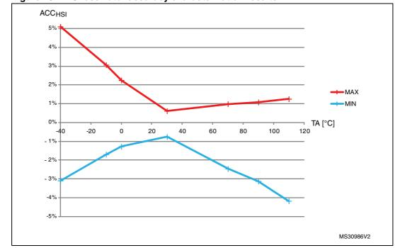
Figure 16. HSI oscillator accuracy characterization results
