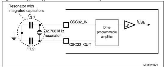
Figure 15. Typical application with a 32.768 kHz crystal
