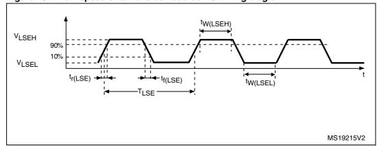
Figure 13. Low-speed external clock source AC timing diagram
