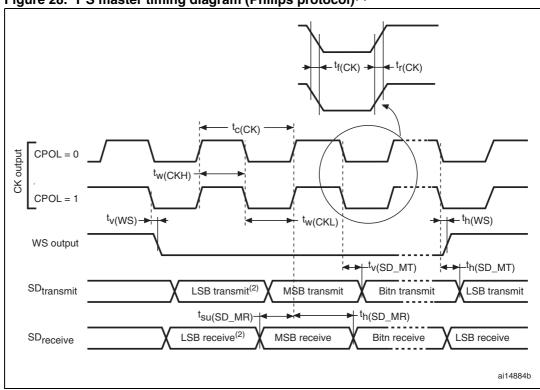
Figure 28. I<sup>2</sup>S master timing diagram (Philips protocol)<sup>(1)</sup>
