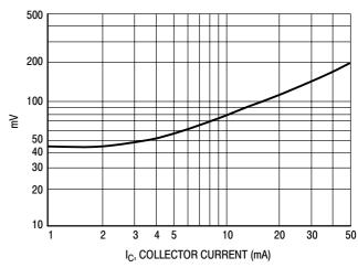
Figure 2.  $V_{CE(sat)}$  at  $I_C/I_B = 10$
