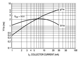
Figure 5. Input Impedance at 30 MHz
