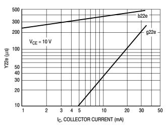
Figure 6. Output Impedance at 30 MHz
