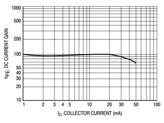
Figure 1. h<sub>FE</sub> at 10 V
