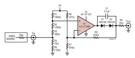
Figure 10. Single Supply RGB Video Amplifier (1 of 3 Channels)
