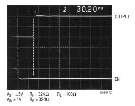
Figure 2. Amplifier Enable Time,  $A_V = 2$
