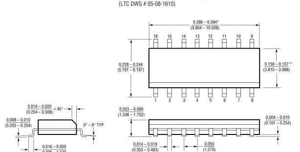
\*DIMENSION DOES NOT INCLUDE MOLD FLASH. MOLD FLASH SHALL NOT EXCEED 0.006" (0.152mm) PER SIDE
