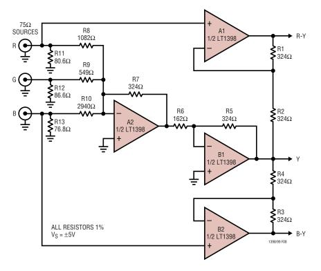
Figure 8. Buffered RGB to Color-Difference Matrix
