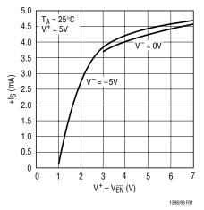
Figure 1.  $+I_S$  vs  $(V^+ - V_{EN})$
