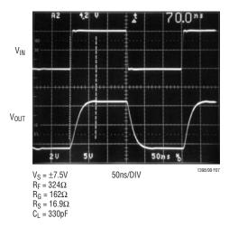
Figure 7. LT1399HV Output Voltage Swing
