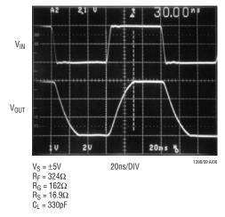
Figure 6. LT1399/LT1399HV Large-Signal Pulse Response
