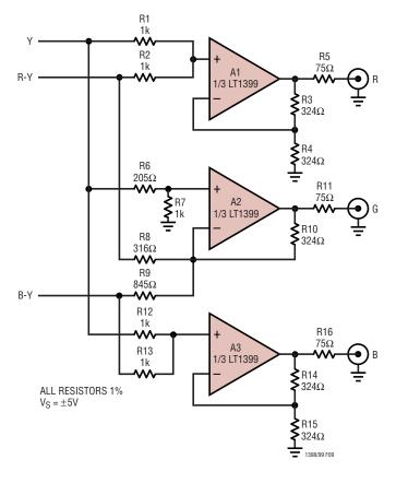
Figure 9. Buffered Color-Difference to RGB Matrix
