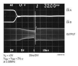
Figure 5. 3-Input Video MUX Switching Response ( $A_V = 2$ )
