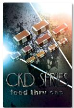
TDK Feed Through CKD series capacitors feature 3-terminal design with even lower ESL than Flip Type capacitors. Feed through design consists of 3-terminal construction where the 3rd terminal acts as a ground. Unique internal design allows for low parallel inductance and offer excellent noise reduction capability for high speed digital IC decoupling.
