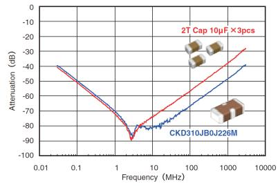
➤ It is possible to reduce the number of components with CKD Series capacitor because one CKD part has similar or better attenuation characteristics as three standard 2-terminal capacitors.
