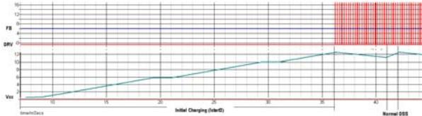
Figure 3. Initial Charging of V<sub>CC</sub> and Normal DSS
