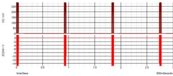
**Figure 12. Output Short Detection and Protection Waveform**
