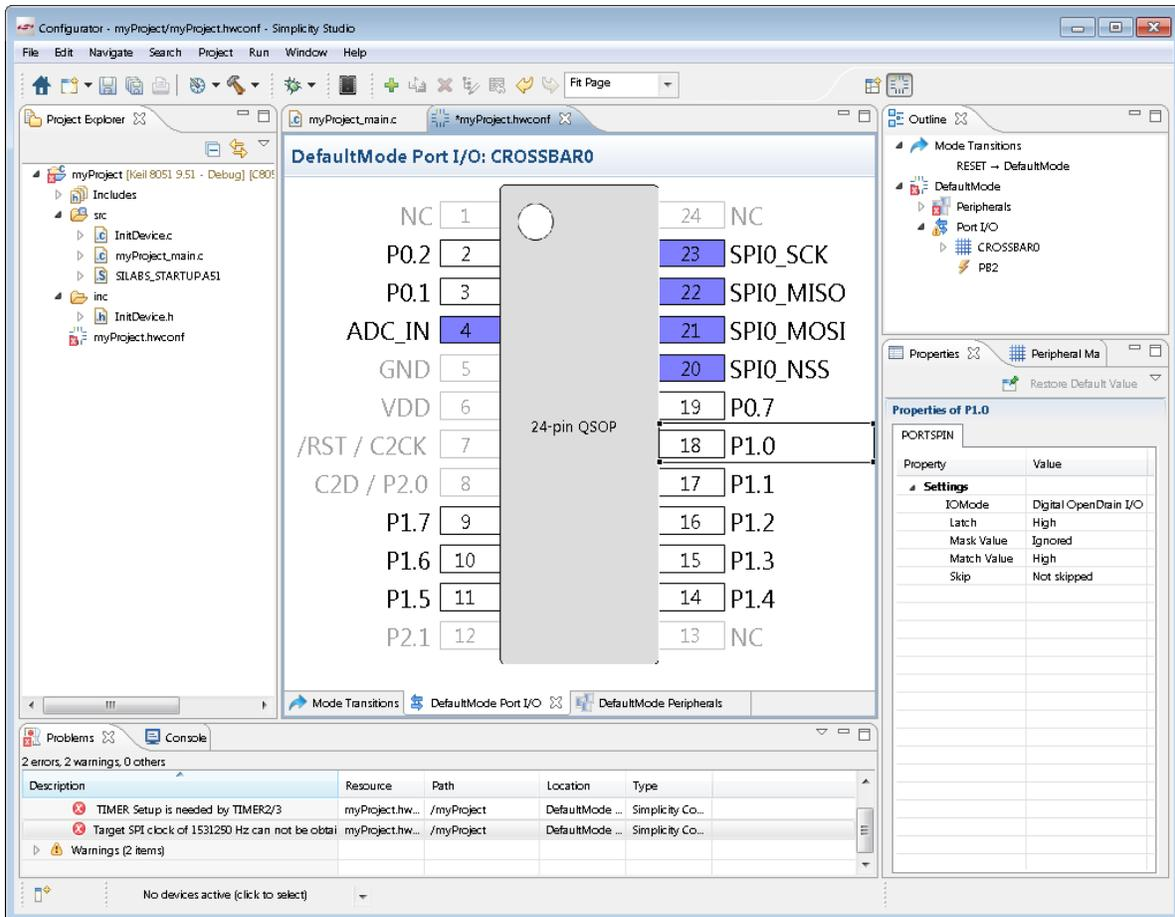
Figure 6. Simplicity Configurator – Configuring Port I/O
