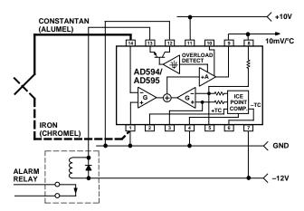
Figure 12. -ALM Driving A Negative Referenced Load
