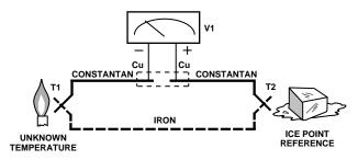
Figure 14. Thermocouple Voltage with 0°C Reference
