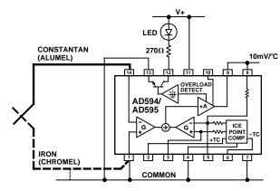
Figure 11. Alarm Directly Drives LED
