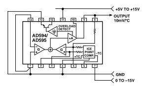
Figure 13. AD594/AD595 as a Stand-Alone Celsius Thermometer
