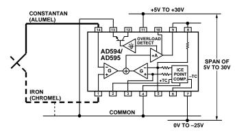
Figure 2. Dual Supply Operation
