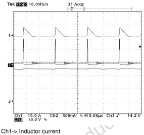
Ch2-> Output voltage Ch3-> Phase voltage
