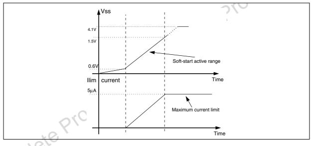
Because the system implements the soft start controlling the inductor current, the soft start capacitor selection is function of the output capacitance, the current limit and the soft start active range ( $\Delta V_{SS}$ ).
