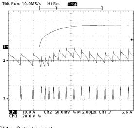
Ch1-> Output current Ch2-> Output voltage Ch3->Phase voltage
