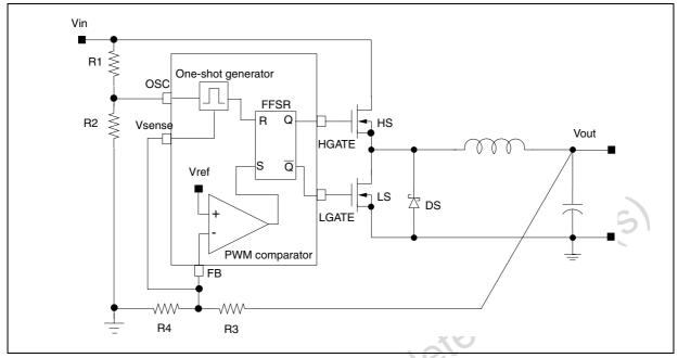
The device implements a Constant On Time control scheme, where the Ton is the high side MOSFET on time duration forced by the one-shot generator. The on time is directly proportional to VSENSE pin voltage and inverse to OSC pin voltage as in Eq1:
