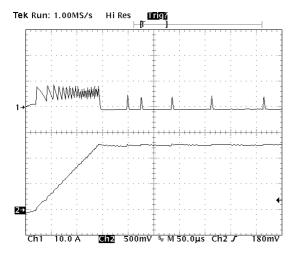
Ch1-> Inductor current Ch2-> Output voltage
