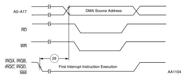
Figure 3-8 External Memory Access (DMA Source) Timing
