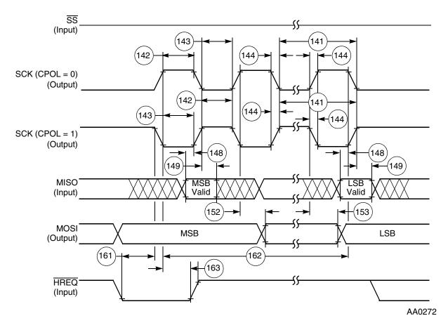
Figure 3-28 SPI Master Timing (CPHA = 1)
