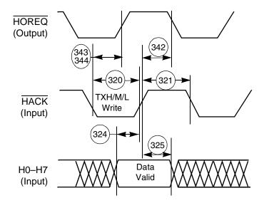
Figure 3-25 Host DMA Write Timing Diagram
