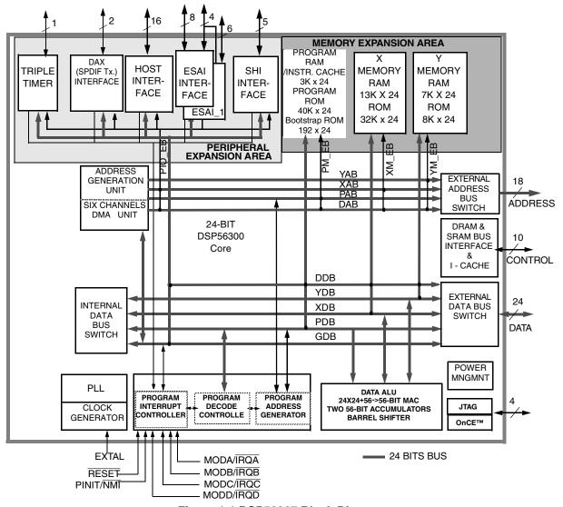
Figure 1-1 DSP56367 Block Diagram
