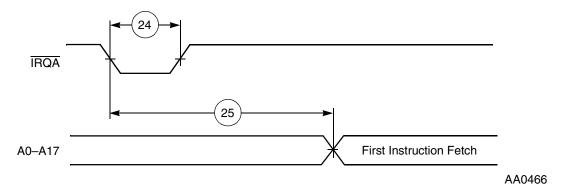
Figure 3-6 Recovery from Stop State Using IRQA Interrupt Service
