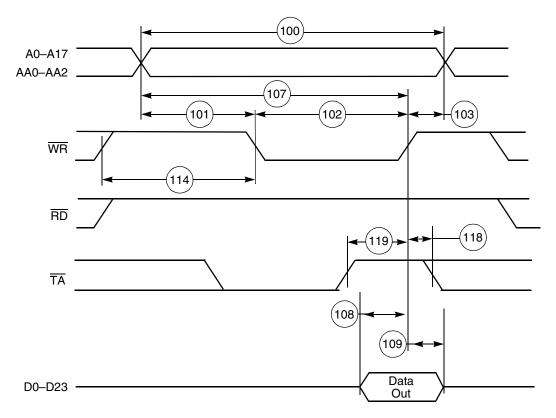
Figure 3-10 SRAM Write Access
