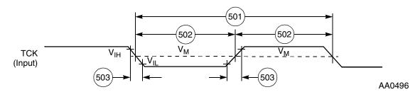
Figure 3-39 Test Clock Input Timing Diagram
