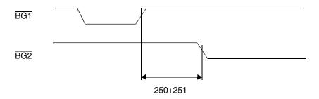
Figure 3-19 Asynchronous Bus Arbitration Timing
