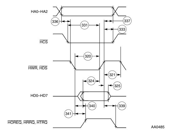
Figure 3-22 Write Timing Diagram, Non-Multiplexed Bus
