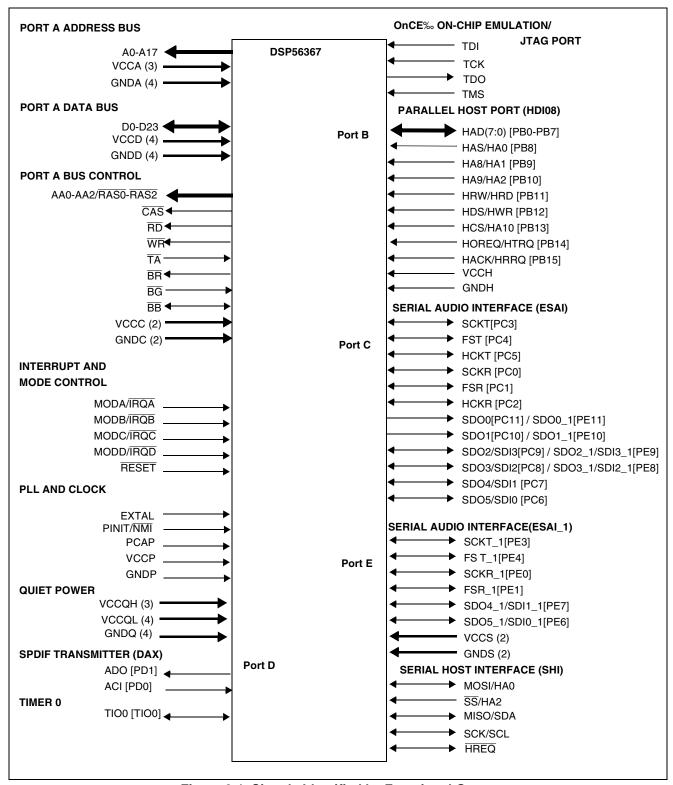
Figure 2-1 Signals Identified by Functional Group
