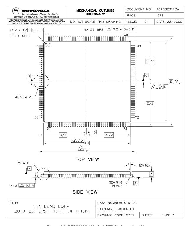
Figure 4-2 DSP56367 144-pin LQFP Package (1 of 3)
