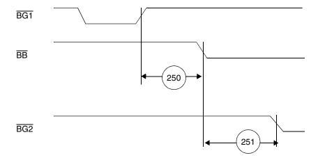
Figure 3-18 Asynchronous Bus Arbitration Timing
