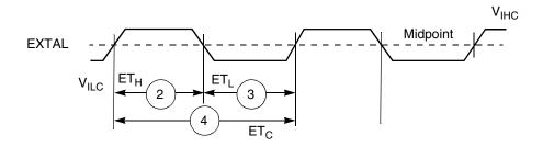
Note: The midpoint is 0.5  $(V_{IHC} + V_{ILC})$ .
