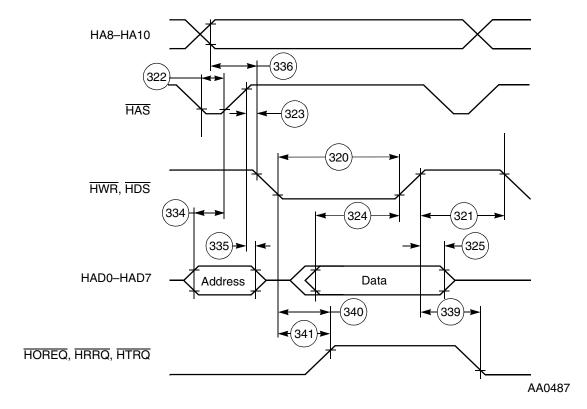
Figure 3-24 Write Timing Diagram, Multiplexed Bus
