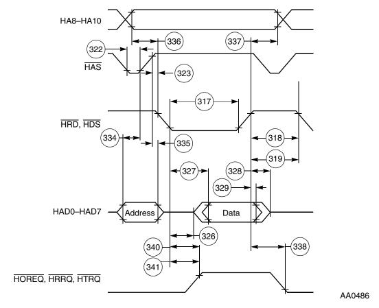
Figure 3-23 Read Timing Diagram, Multiplexed Bus
