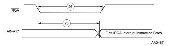
Figure 3-7 Recovery from Stop State Using IRQA Interrupt Service
