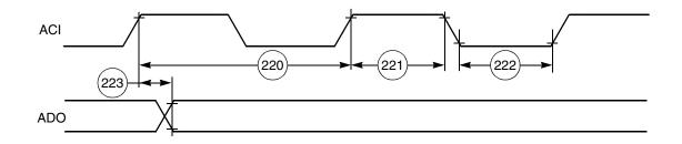
Figure 3-36 Digital Audio Transmitter Timing
