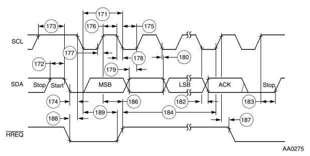
Figure 3-31 I<sup>2</sup>C Timing
