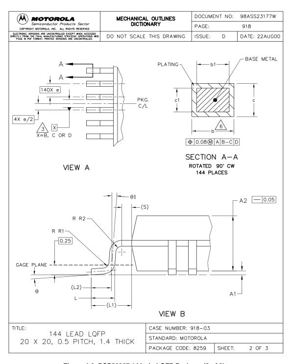
Figure 4-3 DSP56367 144-pin LQFP Package (2 of 3)
