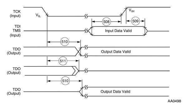
Figure 3-41 Test Access Port Timing Diagram
