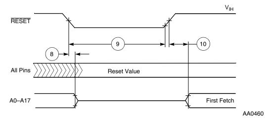
Figure 3-2 Reset Timing
