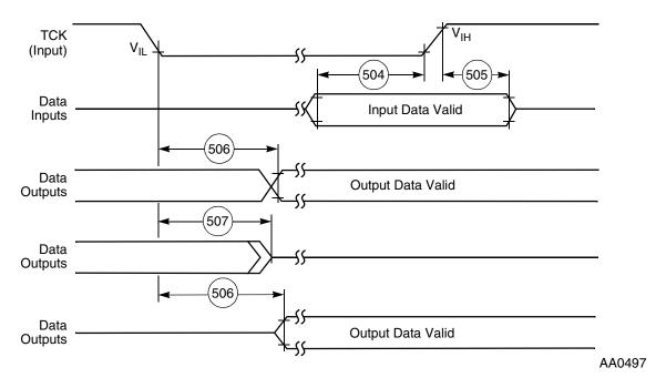
Figure 3-40 Boundary Scan (JTAG) Timing Diagram
