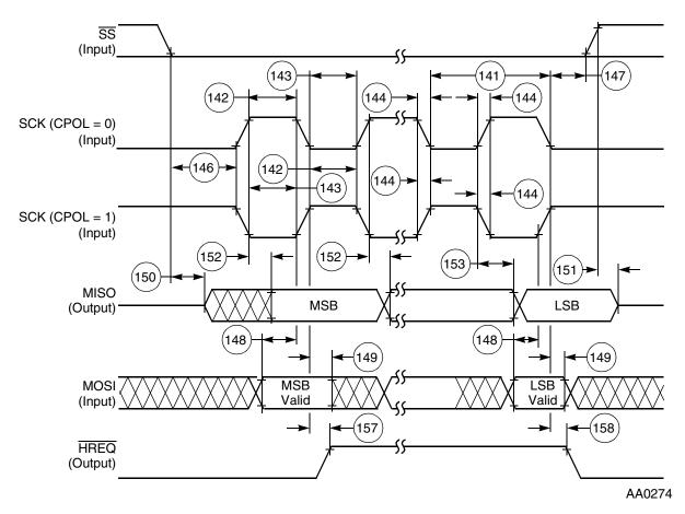
Figure 3-30 SPI Slave Timing (CPHA = 1)
