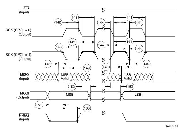
Figure 3-27 SPI Master Timing (CPHA = 0)
