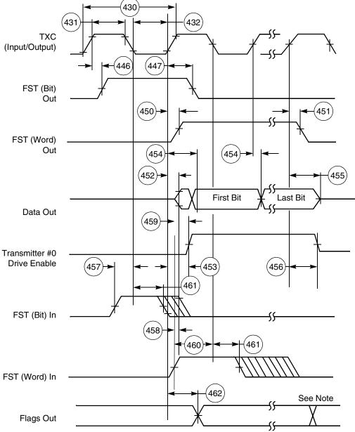
Note: In network mode, output flag transitions can occur at the start of each time slot within the frame. In normal mode, the output flag state is asserted for the entire frame period.
