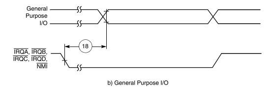
Figure 3-3 External Fast Interrupt Timing
