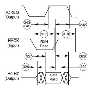
Figure 3-26 Host DMA Read Timing Diagram
