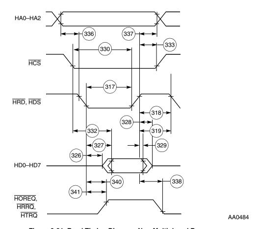
Figure 3-21 Read Timing Diagram, Non-Multiplexed Bus
