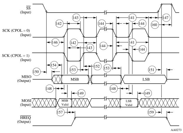
Figure 3-29 SPI Slave Timing (CPHA = 0)
