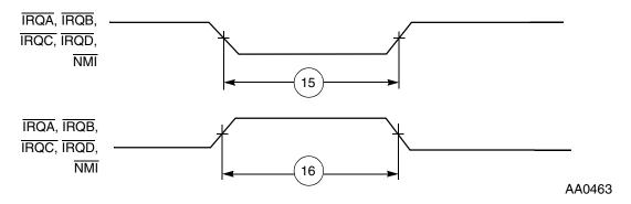
Figure 3-4 External Interrupt Timing (Negative Edge-Triggered)
