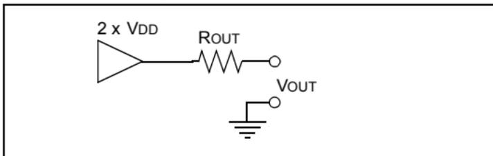
To design a voltage doubler, first determine the maximum tolerable output resistance based on the required output current and the minimum tolerable output voltage. Remember that the output current will be limited to one half of the output capability of the comparator. Then choose a transfer capacitance and switching frequency using Equation 10-1.
