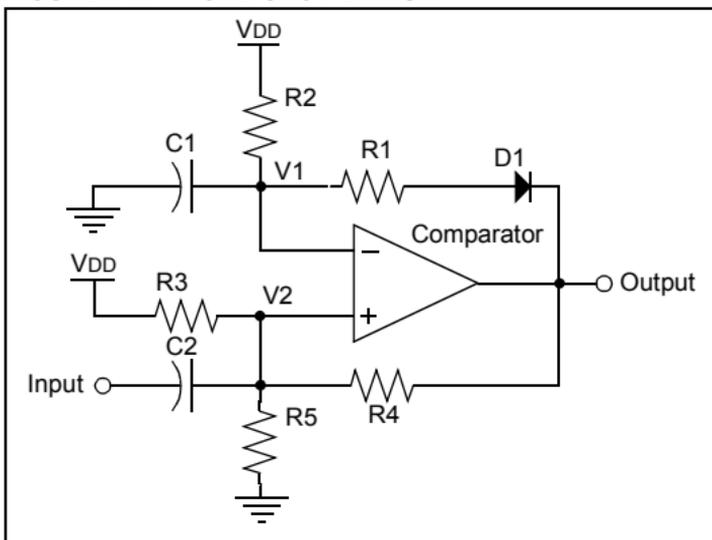
To design the one-shot, first create the hysteresis feedback using the techniques from TIP #3. Remember to set the low threshold below 0.7V. Next, choose values for R2 and C1 using Equation 7-1.
