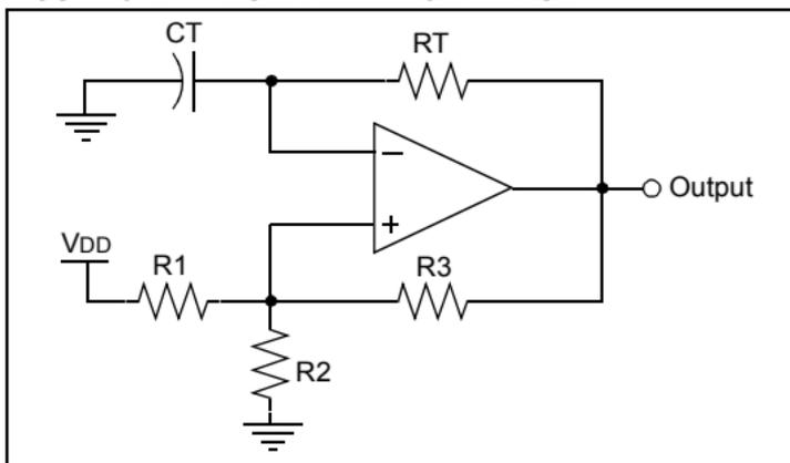
To design a multi-vibrator, first design the hysteresis feedback path using the procedure in TIP #3. Be careful to choose threshold voltages ( $V_{TH}$  and  $V_{TL}$ ) that are evenly spaced within the common mode range of the comparator and centered on  $V_{DD}/2$ . Then use  $V_{TH}$  and  $V_{TL}$  to calculate values for  $R_T$  and  $C_T$  that will result in the desired oscillation frequency  $F_{OSC}$ .
