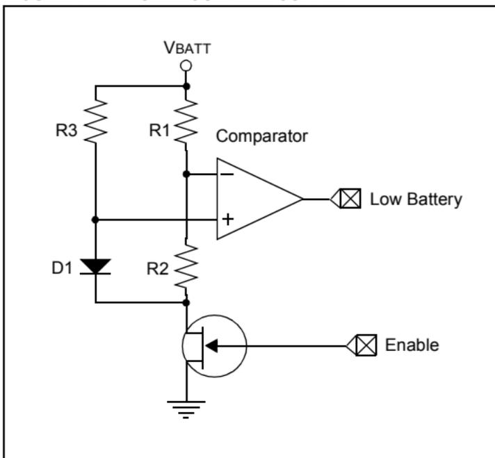
Comparator will trip when  $V_{BATT} = 3V$ :  $R1 = 33k$ ,  $R2 = 10k$  and  $R3 = 470\Omega$ .
