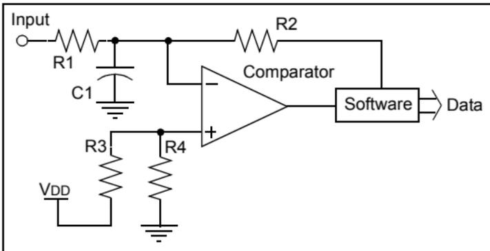
In operation, the feedback output from the software is a time sampled copy of the comparator output. In normal operation, the modulator output generates a PWM signal which is inversely proportional to the input voltage. As the input
