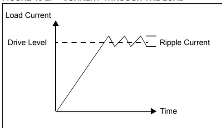
To design a PWM high current driver, first determine a switching speed ( $F_{SWX}$ ) that is appropriate for the system. Next, choose a MOSFET and D1 capable of handling the load current requirements. Then choose values for  $R_2$  and  $C_1$  using Equation 13-1.
