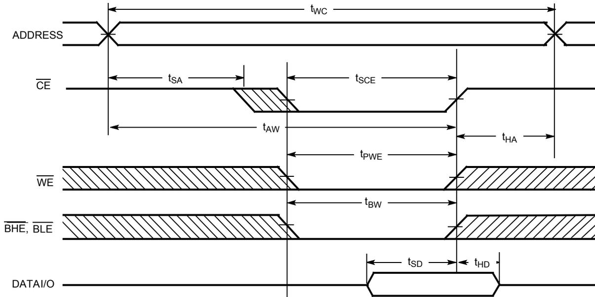
Figure 7. Write Cycle No. 2 ( $\overline{\text{BLE}}$  or  $\overline{\text{BHE}}$  Controlled)
