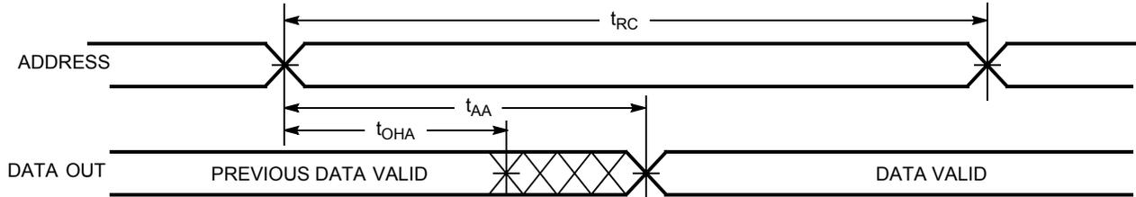
Figure 5. Read Cycle No. 2 ( $\overline{OE}$  Controlled) [12, 13]
