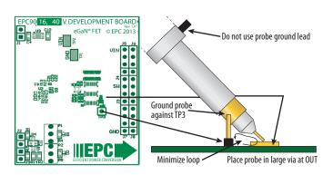
Figure 3: Proper Measurement of Switch Node  $-V_{\text{SW}}$
