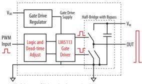
Figure 1: Block Diagram of EPC9016 Development Board
