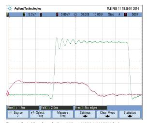
Figure 4: Typical Waveforms for V $_{IN}=24\,V$  to 1.2 V/25 A (1000kHz) Buck converter CH2: Switch node voltage (Vsw) — CH4: PWM input voltage (V $_{PWM}$ )
