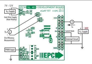
Figure 2: Proper Connection and Measurement Setup
